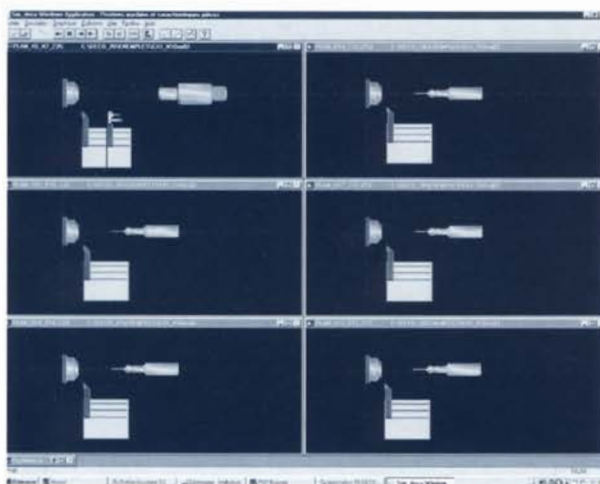
Sim Deco Version 4.0, the simulation program of the tool path
